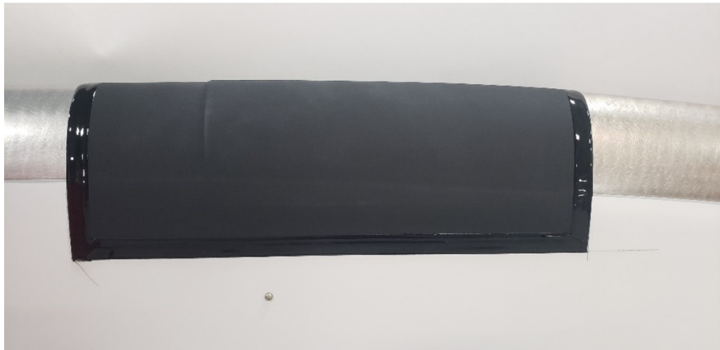
Figure 3 ~ Completed Polyurethane Tape Installation – Tip Abrasion Strip Joint
